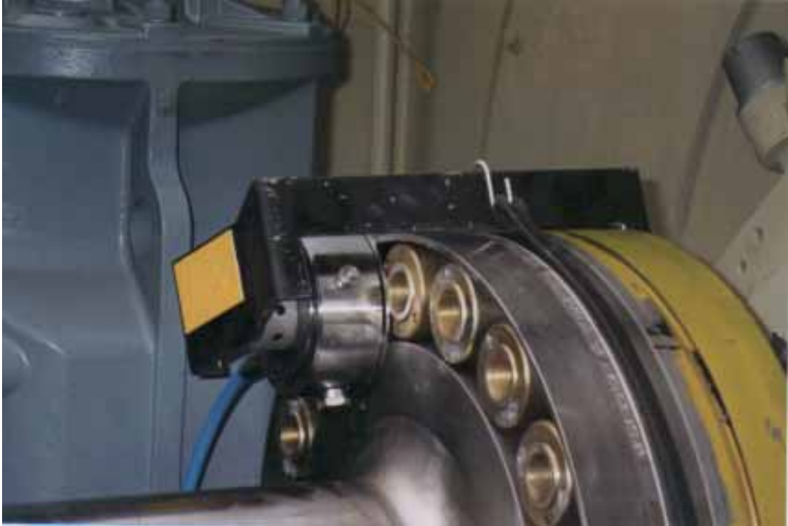
Photo 2 Side view of 2" puller tool and safety cage on 6FA machine.
